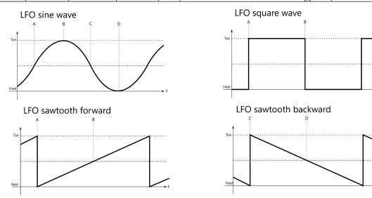
The LFO starts immediately at the specified starting point. Resending the commands will reset the engine to start over from the starting point.
