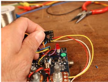
Now some functions can be tested. Be careful, that the Goblin and the Pitch Fork aren't touching and plug in the power supply. The red LED of the Goblin should light up. Check if the bypass switch and the Shift and Blend knobs are working.
