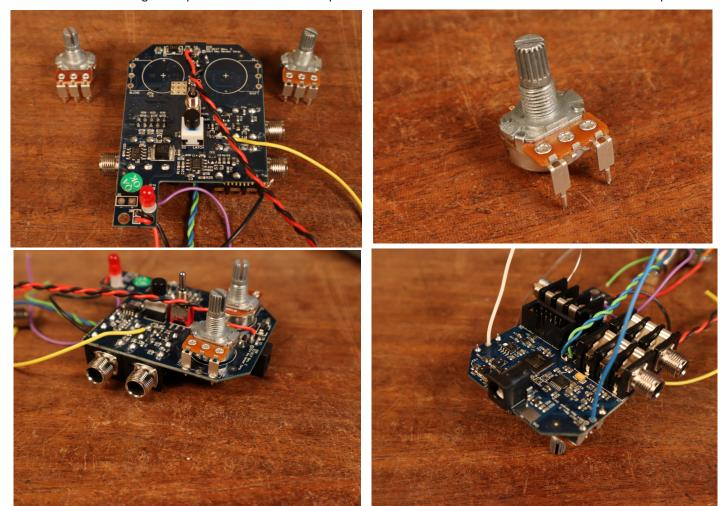
Then wires are soldered to the place where the potentiometer legs were in the circuit board (blue and white in the picture). Also two wires are soldered to the place were the potentiometer legs were cut off (yellow and orange in the picture). After that a last wire is needed for the reference voltage. This is soldered somewhere where there is 3.3V, like on the top leg of the blend knob, like the red wire in the picture on the bottom left.
