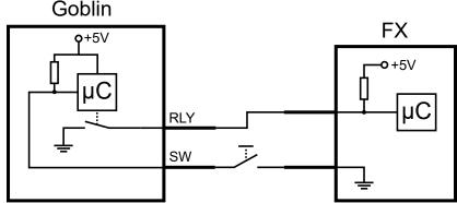
Before connecting the Goblin it is important to control, that the voltage on the effects device does not exceed 5V. Below is fine.
