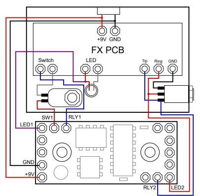
Effects Device with Foot Switch and External TRS Connector with Goblin-EXP
