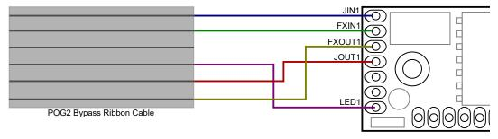
Connect the wires from step 3, 4 and 5 like this:
